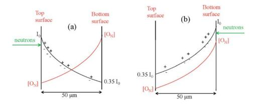
FIG. 2. Schematic illustrations of the  $O_N$  defect (oxygen impurities occupying nitrogen sites) distribution and radiation-generated charge carriers inside  $h^{-10}BN$  detectors for radiation entered from the (a) top surface and (b) bottom surface.
