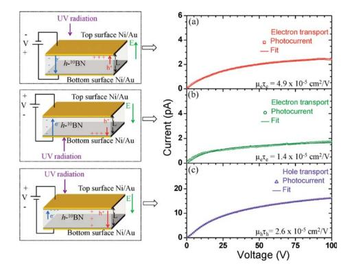
FIG. 5. Photocurrent-voltage characteristics measured under UV radiation for three different device configurations.
