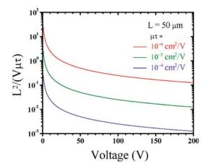
FIG. 6. Plot of  $L^2/(V\mu\tau)$  vs. bias voltage (V) for  $\mu\tau = 10^{-6}$ ,  $10^{-5}$ , and  $10^{-4}$  cm<sup>2</sup>/V for 50  $\mu$ m thick h-<sup>10</sup>BN detectors.
