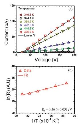
FIG. 8. (a) Dark I-V characteristics measured for the device configuration shown in Fig. 3(a) at different temperatures, from which the temperature dependence of the sample resistance (R) can be extracted. (b) An Arrhenius plot of R, ln (R) vs 1/T, and the solid line is a linear fit.
