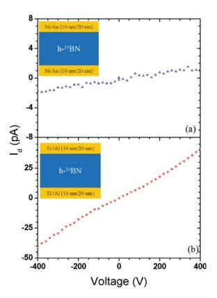
FIG. 4. Dark I-V characteristics measured for the device configuration shown in (a) Fig. 3(a) and (b) Fig. 3(b).
